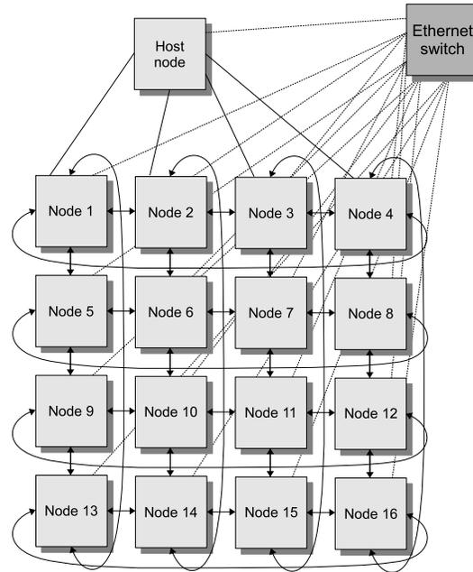
**Fig. 1.5** Architecture of the cluster used in tests.
