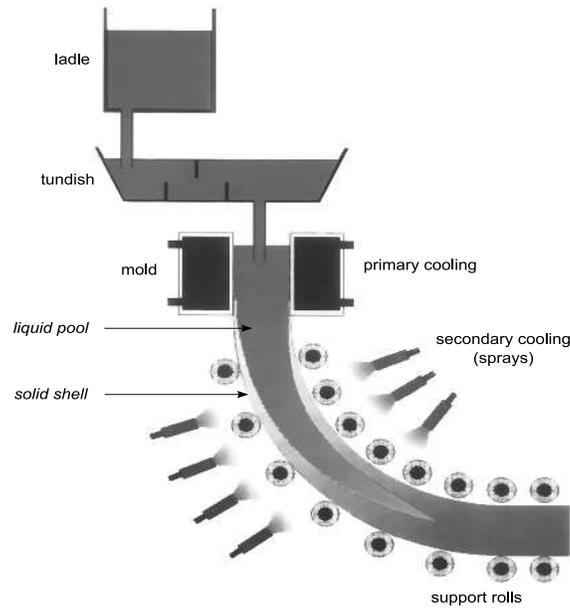
**Fig. 1.4** A schematic view of continuous casting of steel.
