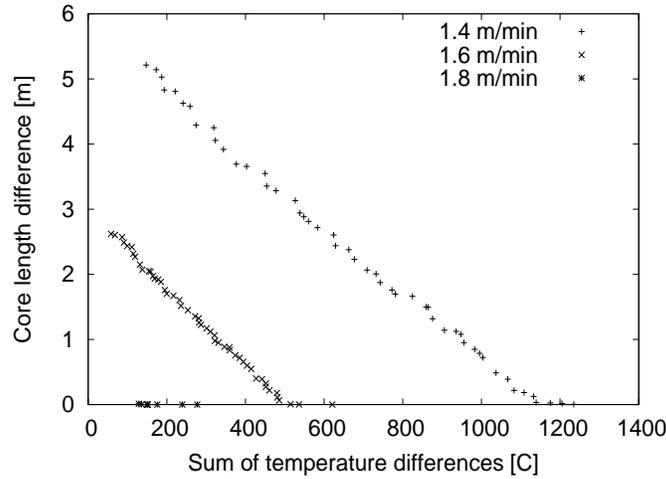
**Fig. 1.6** Nondominated fronts of solutions to the two-objective steel casting optimization problem for various casting speeds.
